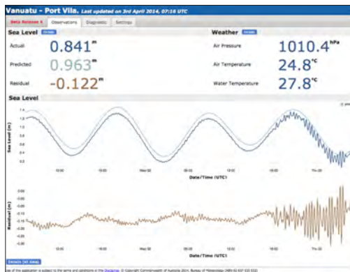
Real-time display on 4 April 2014 for Port Vila, Vanuatu, clearly shows the spread of waves from the Chilean tsunami.
